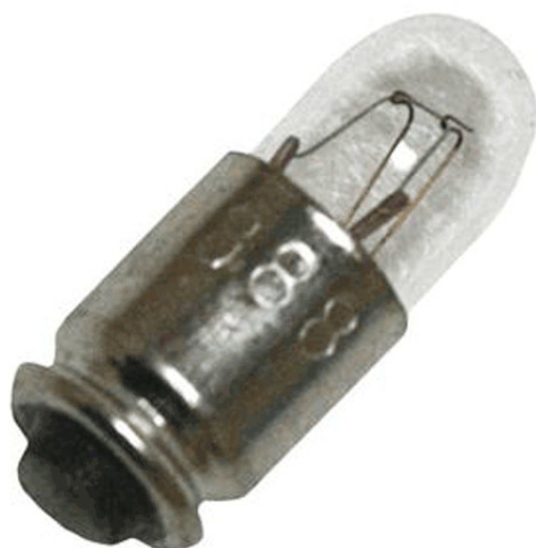
T1 3/4 Midget Grooved 24V 35mA 10KH
