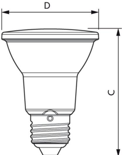
E27 PAR20 Led MASTER LEDspot 6w = 50W 927
