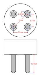
G10Qb Tube 12GPM55 TUV UVC 940mm 4 pins 253.7nm
