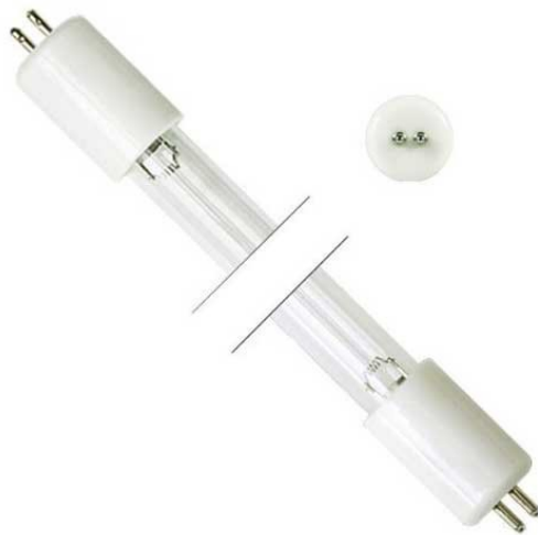
Tube germicide UVC ZW30S19W-Z894 30w 894/910mm 2 pins
