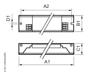
Ballast electronique HF-P 158 TL-D III 220-240V 50/60Hz IDC
